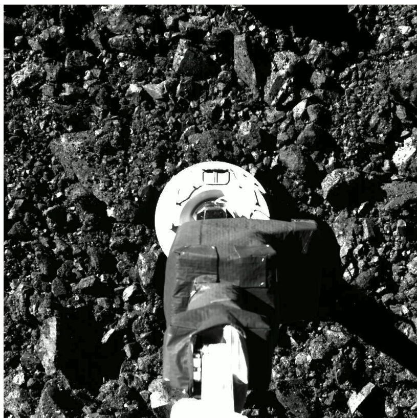
Captured on Oct. 21 AEST during the OSIRIS-REx mission's Touch-And-Go (TAG) sample collection event, this image shows the SamCam imager's field of view at the moment after the NASA spacecraft touched down on asteroid Bennu's surface. The sampling event brought the spacecraft all the way down to sample site Nightingale, and the team on Earth received confirmation of successful touchdown at 6:08 p.m. EDT. Preliminary data show the sampling head touched Bennu's surface for approximately 6 seconds, after which the spacecraft performed a back-away burn.
